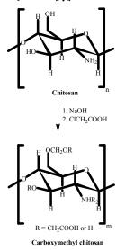
Fig. 2. Preparation of carboxymethyl chitosan
