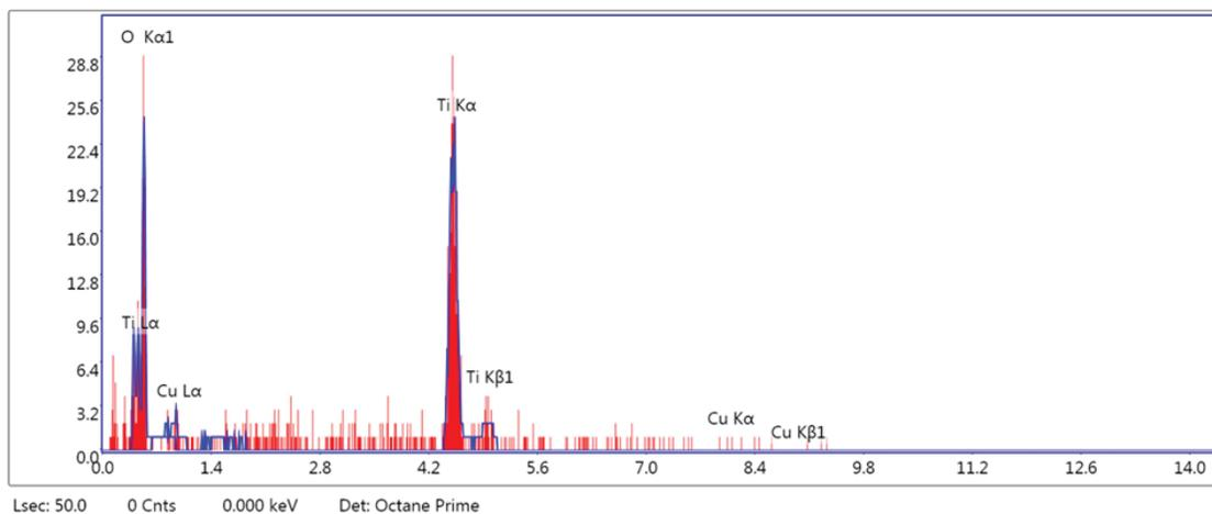
**Fig. 3.** EDX spectra of Cu(II) doped  $\text{TiO}_2$  composite.
