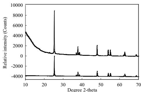
**Fig. 4.** Comparison of XRD pattern of Cu(II) doped  $\text{TiO}_2$  composite (top) and  $\text{TiO}_2$  (bottom).
