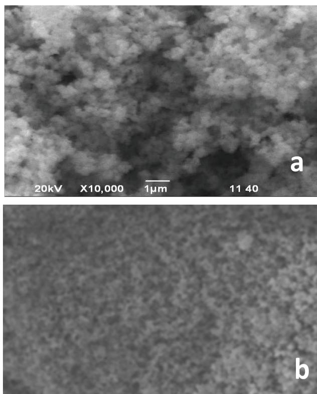
Fig. 2. SEM images of TiO<sub>2</sub> (a) and Cu(II) doped TiO<sub>2</sub> composite (b).
