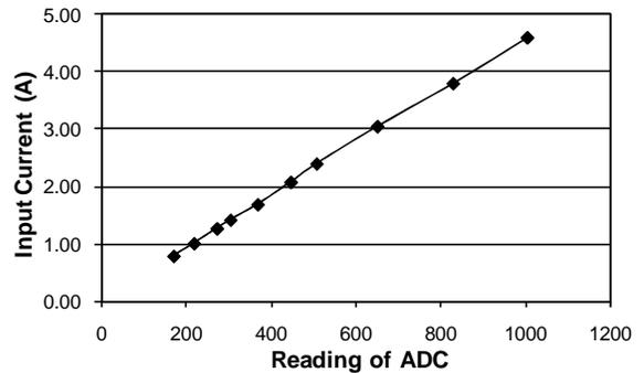
Fig. 11. Graph for calibration of current sensor
