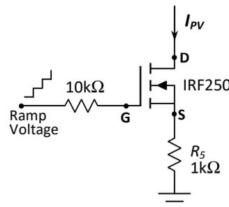
Fig. 4. Active load Circuit
