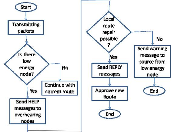
Fig. 11. Proposed route repair process
