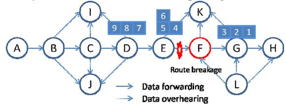
Fig. 12. Route breakage due to node F is down
