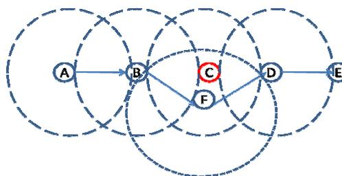
Fig. 2. New route possible using F
