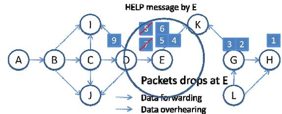
Fig. 13. Packets 7 and 8 are dropped at node E
