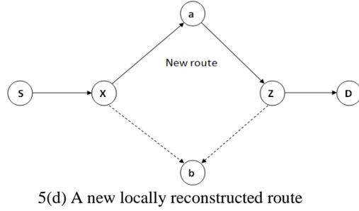
Fig. 5. QLR steps to repair route locally
