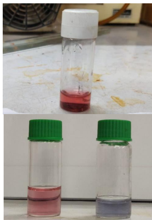
Fig. 1: (a) Pure GNP solution. (b) After the addition of CuCl_2 and H_2O_2 respectively
