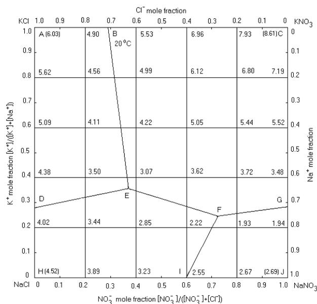
Figure 1: Phase diagram of system ( $K^+$ ,  $Na^+$ ,  $Cl^-$ ,  $NO_3^-$ )- $H_2O$  at  $20^\circ C$  calculated by extended UNIQUAC model. Numbers on intersections and four corners represent moles of  $H_2O$ /total moles of ions
