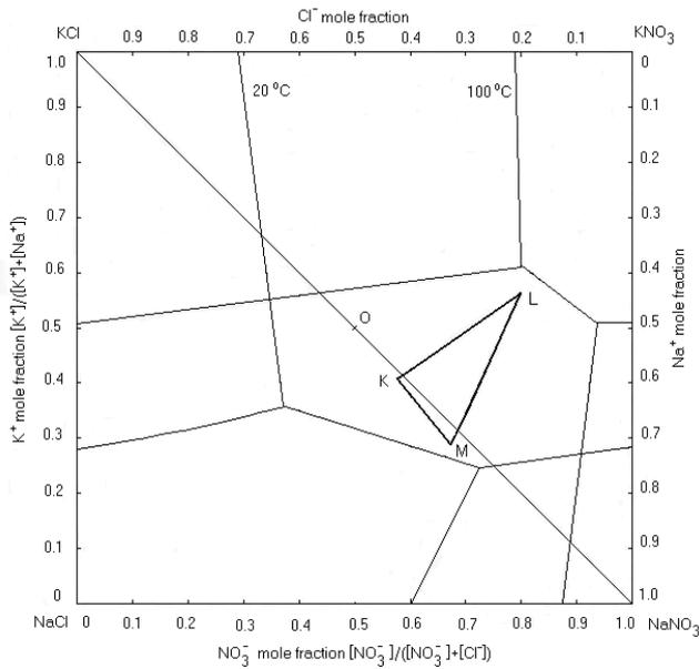
Figure 2: Two isotherms and cyclic process for fractional crystallization of NaCl (at 100°C) and KNO<sub>3</sub> (at 20°C)
