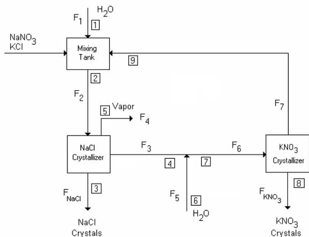
Figure 3: KNO<sub>3</sub> process labeled with total flow rate of streams. The numbers in squares are stream numbers
