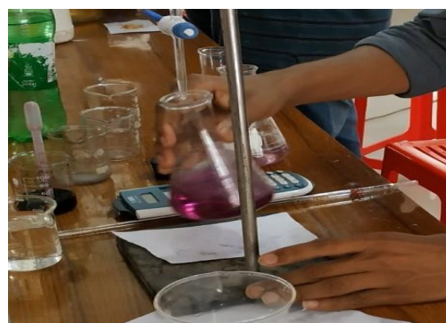
Fig.2: Water Hardness test using EDTA method
