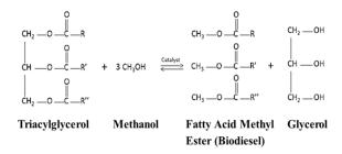
Fig. 1: An illustration of trans-esterification reaction for biodiesel production
