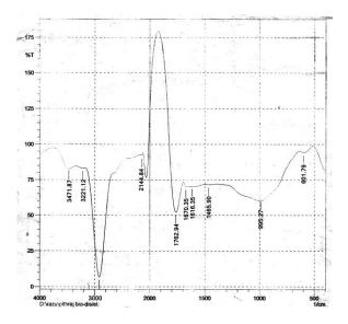
Fig. 4: FTIR spectrum of produced biodiesel from PS oil
