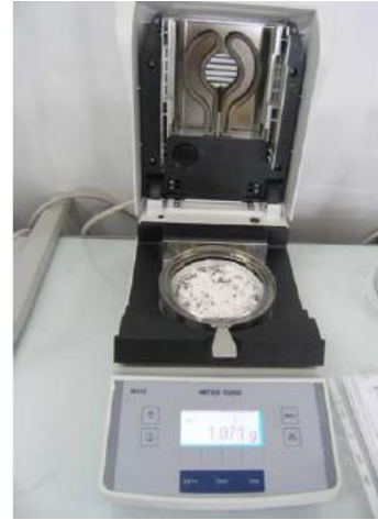
Figure 7: MJ33 Moisture Analyzer with sieved granules loaded.
