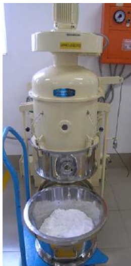
Figure 6: Sapphire Fluid Bed Dryer with wet granules loaded.
