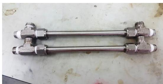
**Figure 1:** Hollow fiber membrane module.
