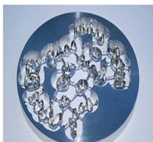
Fig 17: Chrome-cobalt disc with bridges and crowns manufactured using WorkNC Dental CAD-CAM.
