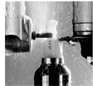
Figure 12: A milling machine located inside the dental office carves a restoration from a block of ceramic material.
