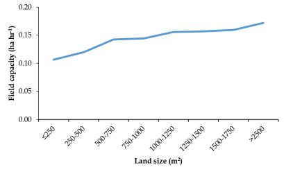
Fig. 4. Field capacity of transplanter with respect to land size. Note: Graph adopted from Islam, 2018a.
