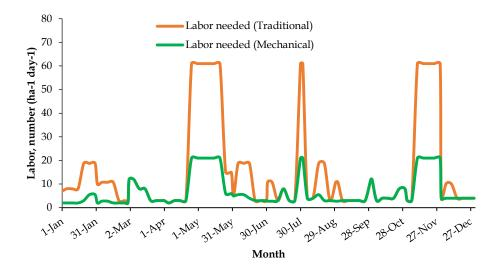
Fig. 2. Labour demand (manual and mechanical) calendar in rice production in Bangladesh. Source: Author calculation based on field survey 2020.
