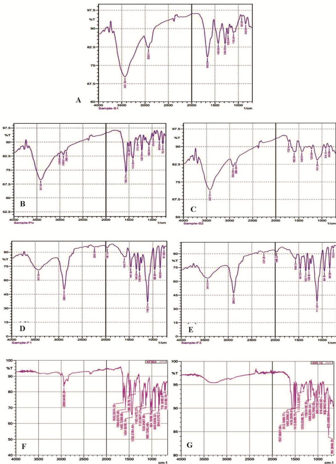
Figure 5. FTIR spectra of (A) PTV, (B) PTV with Kollidon 90F by solvent evaporation (SKN4), (C) PTV with Kollidon 90F by fusion method (FKN4), (D) PTV with Kollicoat IR by solvent evaporation (SKT3), (E) PTV with Kollicoat IR by fusion method (FKT3), (F) PTV with Kollidon 90F by PM method (PKN4), (G) PTV with Kollicoat IR by PM method (PKT3).
