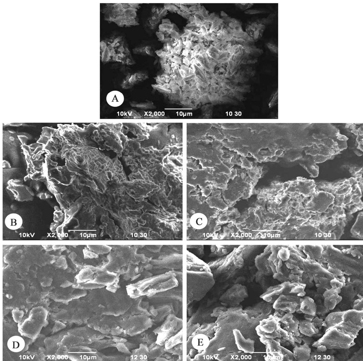
Figure 8. Scanning Electron Microscopic analysis of (A) pure Pitavastatin at X2000 magnification, (B) Pitavastatin with Kollidon 90F prepared by solvent evaporation (SKN4) at X2000 magnification, (C) Pitavastatin with Kollidon 90F prepared by fusion method (FKN4) at X2000 magnification, (D) Pitavastatin with Kollicoat IR prepared by solvent evaporation (SKT3) at X2000 magnification, (E) Pitavastatin with Kollicoat IR prepared by fusion method (FKT3) at X2000 magnification.
