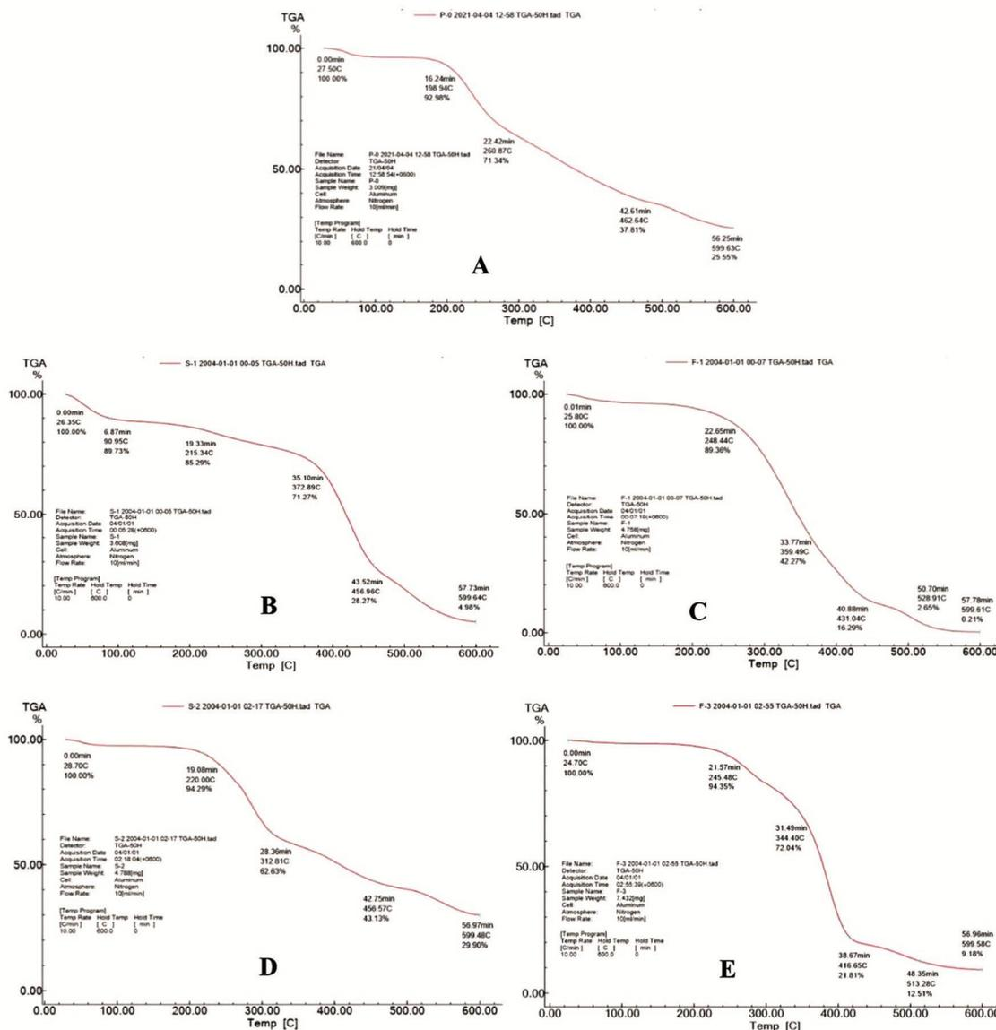
Figure 7. TGA thermograms of (A) PTV, (B) PTV with Kollidon 90F by solvent evaporation (SKN4), (C) PTV with Kollidon 90F by fusion method (FKN4), (D) PTV with Kollicoat IR by solvent evaporation (SKT3), (E) PTV with Kollicoat IR by fusion method (FKT3).
