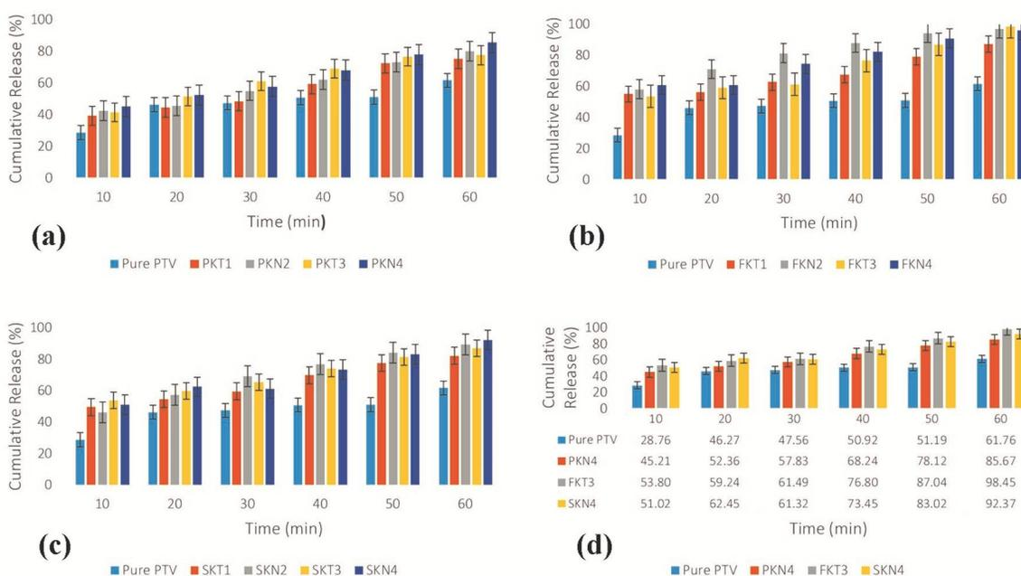
Figure 3. The cumulative percent API release of pure PTV with (a) PM formulations (PKT1, PKN2, PKT3 and PKN4), (b) SD formulations (FKT1, FKN2, FKT3 and FKN4) prepared by fusion method, (c) SD formulations (SKT1, SKN2, SKT3 and SKN4) formulated by solvent evaporation and (d) Comparison among optimized formulations of PMs, SDs and pure PTV.
