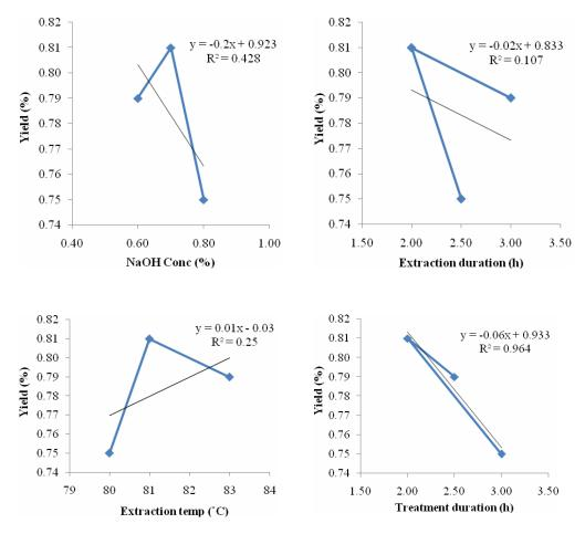
Fig. 5. Relationship between yield (%) of gelatin and the concentration of NaOH (%), extraction duration (hr), extraction temperature (°C) and treatment duration (hr) from the scales of mixed types of scales.
