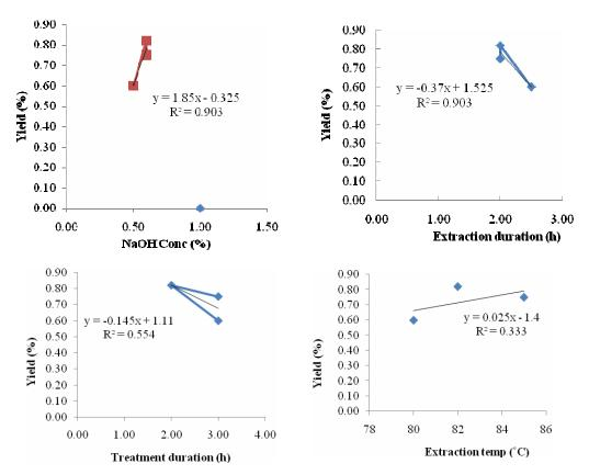
Fig. 2. Relationship between yield (%) of gelatin and the concentration of NaOH (%), extraction duration (hr), extraction temperature (°C) and treatment duration (hr) from the scales of catla.
