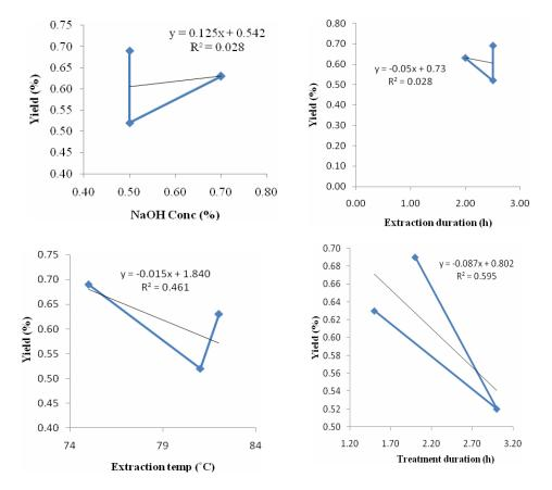
Fig. 3. Relationship between yield (%) of gelatin and the concentration of NaOH (%), extraction duration (hr), extraction temperature (°C) and treatment duration (hr) from the scales of rohu.
