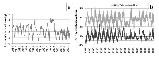
Fig. 2. Long term hydrograph of (a) ground water level below ground surface and (b) surface water level fluctuation curve (Data source BWDB).
