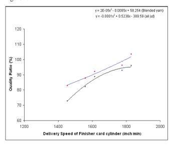
Fig. 1: Quality ratio vs Delevery speed of finisher card cylinder of 275 tex all jute yarn and blended yarn
