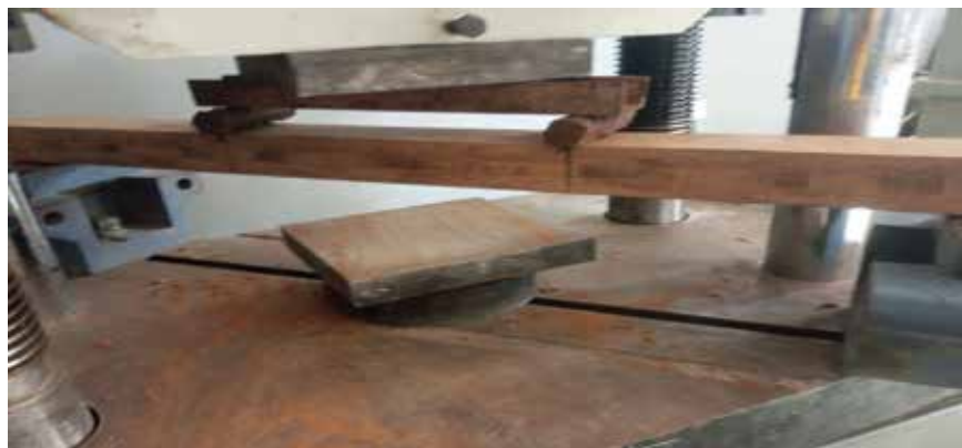
Fig. 3c. 4-Point bending test set-up for solid coconut beams
