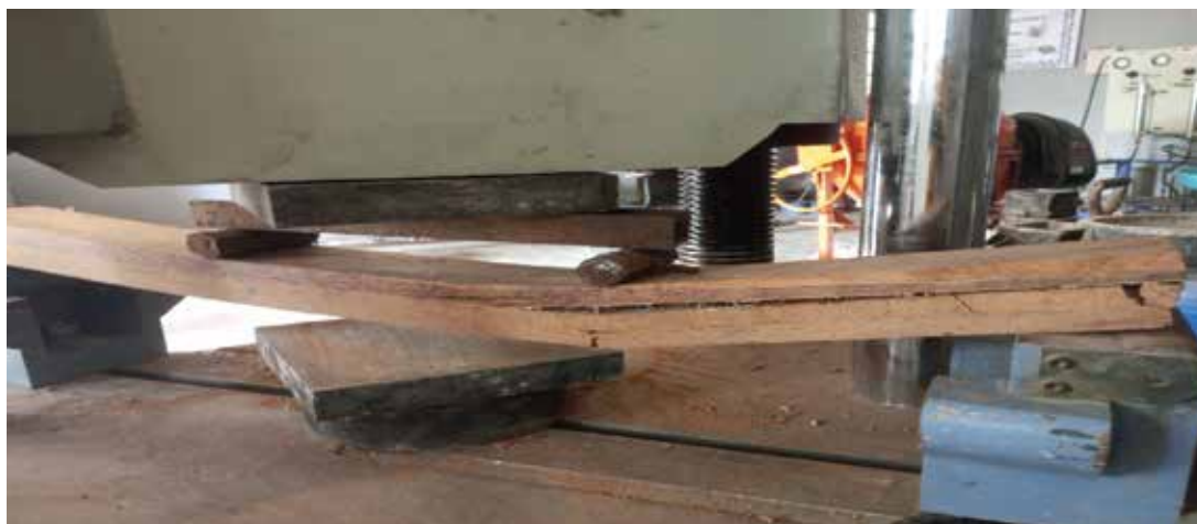
(b) Coconut CLT beam failure
