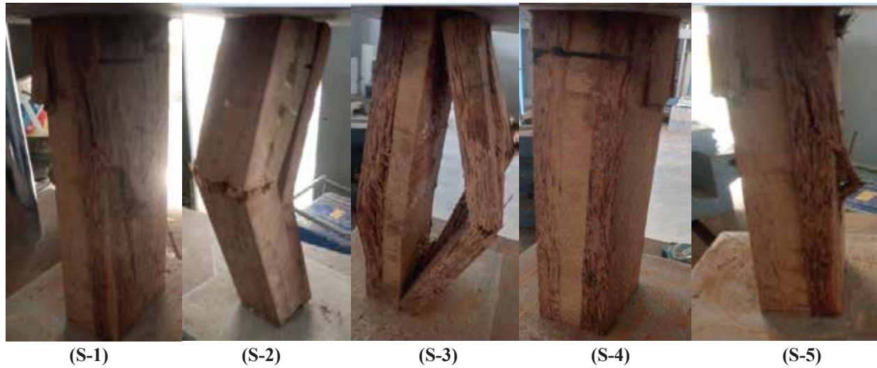
Fig. 9. Solid coconut failure modes
