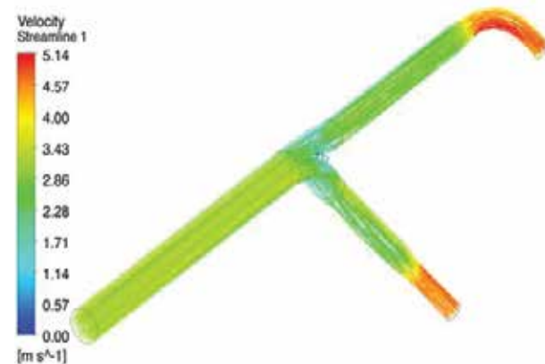
Fig. 12. Velocity streamlines without a sickle in the bifurcation
