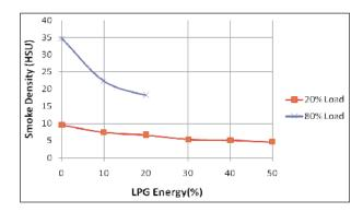
Fig. 6: Variation of Smoke Density with LPG Energy at 20% and 80% Loads
