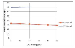
Fig. 3: Variation of Mechanical Efficiency with LGP Energy at 20% and 80% Loads
