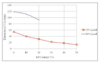
Fig. 9: Variation of Emissions of NOx with LPG Energy at 20% and 80% Loads
