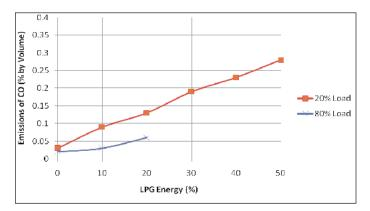
Fig. 8: Variation of Emissions of CO with LPG Energy at 20% and 80% Loads
