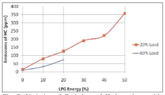
Fig. 7: Variation of Emissions of Hydrocarbons with LPG Energy at 20% and 80% Loads
