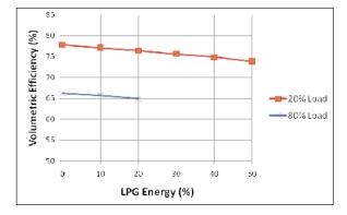
Fig. 4: Variation of Volumetric Efficiency with LPG Energy at 20% and 80% Loads
