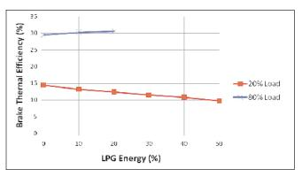
Fig. 2: Variation of Brake Thermal Efficiency with LGP Energy at 20% and 80% Loads
