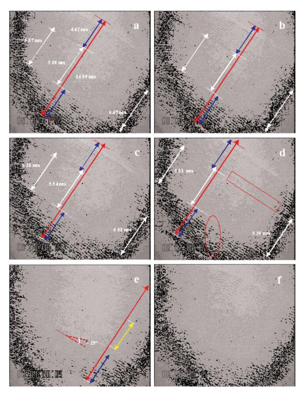
Fig. 3: High resolution transmission electron microscopy (HRTEM) images of an electron irradiated MWCNT (Tube B) with respect to the irradiation exposure time: (a) 7.5 seconds, (b) 15 seconds, (c) 1 minute, (d) 2 minutes and (e) 4 minutes and (f) 8 minutes, respectively
