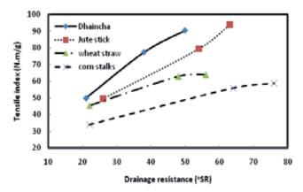
Fig. 2. Tensile index development of KOH pulps with °SR
