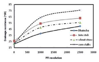
Fig. 1. Increase of drainage resistance of KOH pulps with PFI revolution
