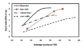
Fig. 4. Burst index development of KOH pulps with °SR
