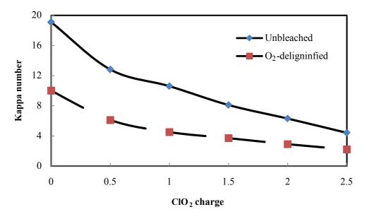
Fig. 1. Effect of chlorine dioxide charge on the D<sub>0</sub>E stage kappa number
