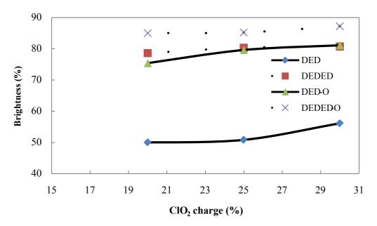
Fig. 2. Final brightness after DED and DEDED sequences of kraft and oxygen delignified pulps
