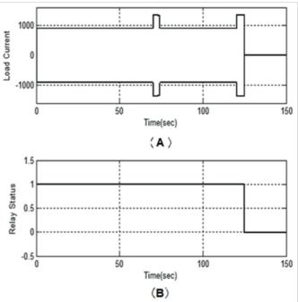
**Fig. 8.(a) The generator output current, (b) Relay status** "Figure 9" illustrated the integrator of frequency relays from 70<sup>th</sup> to 74<sup>th</sup> second, which its time is not 5 seconds, and the relay output does not open the breaker of the generator. But in the 120<sup>th</sup> second the output of integrator takes long more than 5 seconds. The output of relay is issued to the breaker of the generator and separates the generator from the grid.
