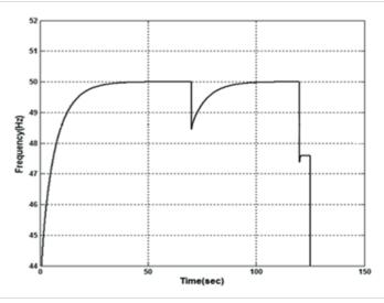
Fig. 5. The grid frequency curve while adding charges
