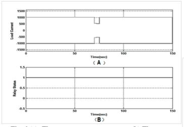
Fig. 6.(a) The generator output current, (b) The status of the relay
