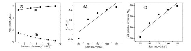
Fig. 2. (a) Plots of cathodic peak current (i) and anodic peak current (ii) as a function of square root of scan rate, (b) Peak current ratio  $(i_{pa2}/i_{pc2})$  dependence on scan rate and (c) A plot of peak potential separation with scan rate for 1.0 mM Cu(II) at pH 3.5.
