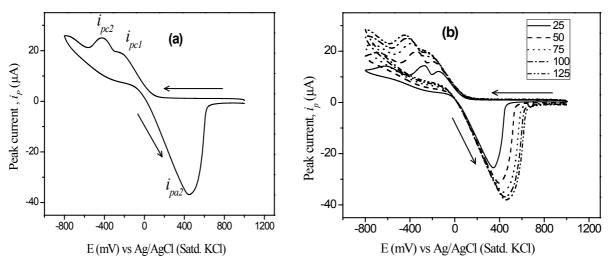
Fig. 1. (a) CV of 1.0 mM Cu(II) in acetate buffer solution at pH 3.5 with scan rate of 100 mVs<sup>-1</sup> and (b) CVs of 1.0 mM Cu(II) at various scan rate: 25 (solid), 50 (dash), 75 (dot), 100 (dash dot), and 125 (dash dot dot) mVs<sup>-1</sup> at GCE.
