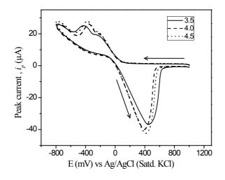
Fig. 3. CVs of 1.0 mM Cu(II) in acetate buffer solution at pH 3.5 (solid), pH 4.0 (dash) and pH 4.5 (dot).
