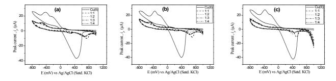
Fig. 6. CVs of Cu(II) (solid), and Cu(II)/Eso with different ratio (i) 1:1 (dash), (ii) 1:2 (dot), (iii) 1:3 (dash dot), and (iv) 1:4 (dash dot dot) in acetate buffer solution at (a) pH 3.5, (b) pH 4.0 and (c) pH 4.5.
