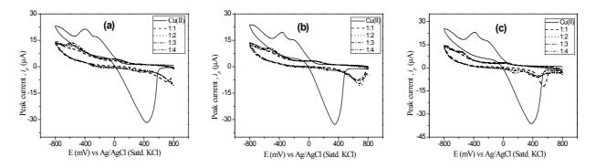
Fig. 4. CVs of Cu(II) (solid), and Cu(II)/Ome with different ratio (i) 1:1 (dash), (ii) 1:2 (dot), (iii) 1:3 (dash dot), and (iv) 1:4 (dash dot dot) in acetate buffer solution at (a) pH 3.5, (b) pH 4.0 and (c) pH 4.5.
