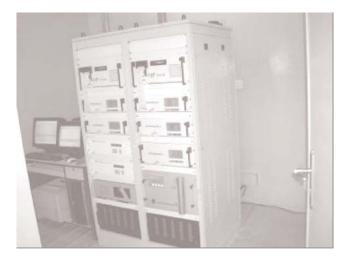
Fig. 1: Multiple Gas analyzers inside of CAMS
