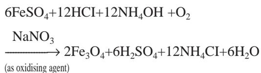
Five series of experiments were performed by varying reaction parameters like amount of hydrochloric acid, type and amount of precipitating agent and oxidizing agent. During these reactions, 100g ferrous sulphate heptahydrate was made 2.5 percent
