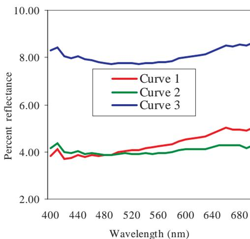
Fig-1: Spectral reflectance curves of some Black Iron Oxide pigment, Curve-1: Sample No-13; Curve-2: Standard Sample and Curve-3: Sample No-13: TiO<sub>2</sub> (5:1).
