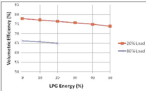
Fig. 4: Variation of Volumetric Efficiency with LPG Energy at 20% and 80% Loads
