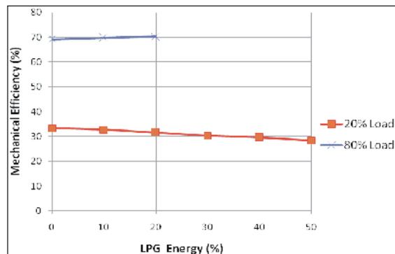
**Fig. 3: Variation of Mechanical Efficiency with LPG Energy at 20% and 80% Loads**
