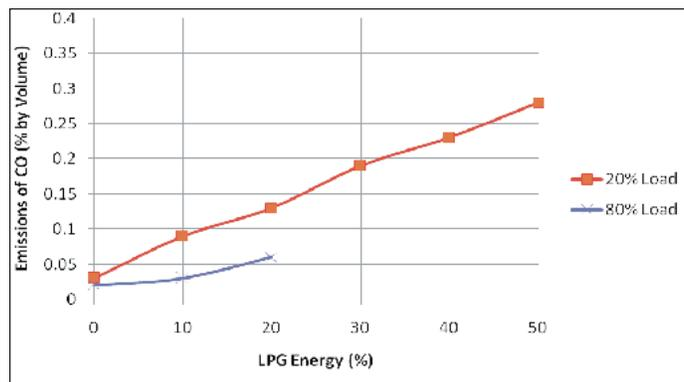
Fig. 8: Variation of Emissions of CO with LPG Energy at 20% and 80% Loads
