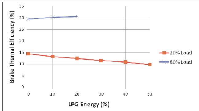
**Fig. 2: Variation of Brake Thermal Efficiency with LPG Energy at 20% and 80% Loads**
