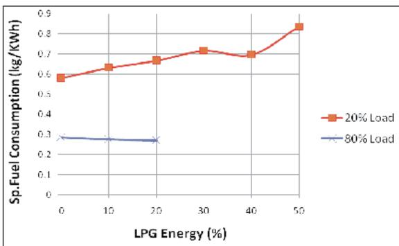
Fig. 5: Variation of Brake Specific Fuel Consumption with LPG Energy at 20% and 80% Loads
