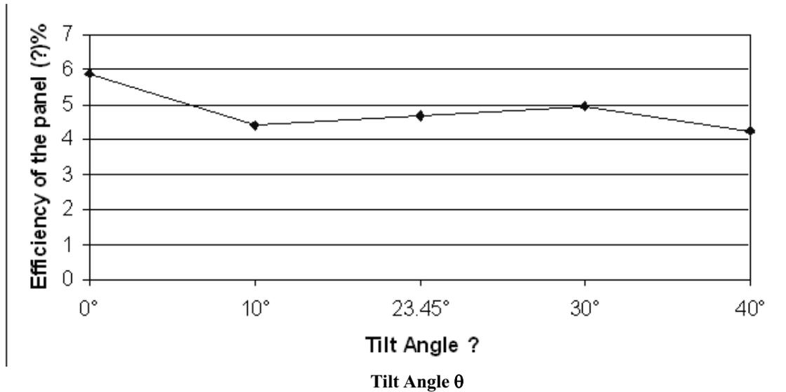
Fig. 1: Variation of efficiencies with tilt angles in summer (June 2006)
