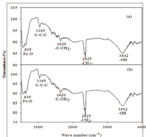
Fig. 2. FTIR spectra of the samples annealed at (a) 250°C and (b) 300°C
