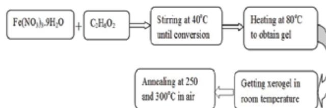
**Fig. 1. Flowchart of synthesis technique of magnetite ( $\text{Fe}_3\text{O}_4$ ) nanoparticles.**
