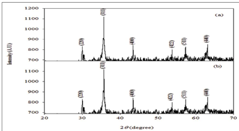
**Fig. 4. XRD patterns of synthesized magnetite annealed at (a) 250°C and (b) 300°C**
