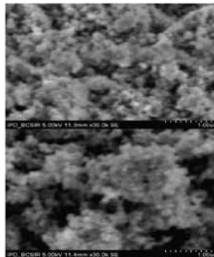
Fig. 3. SEM images of the samples annealed at (a) 250°C and (b) 300°C
