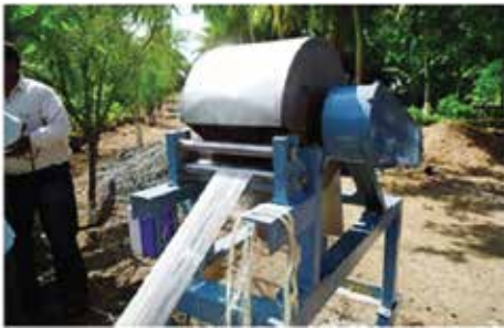
Fig. 1. Photograph of locally fabricated banana fiber extraction machine
