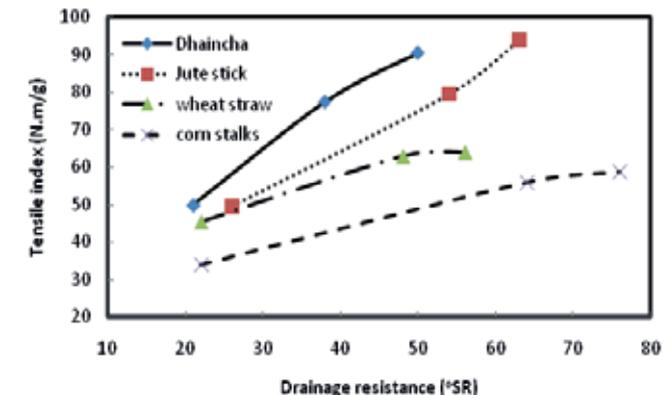
**Fig. 2. Tensile index development of KOH pulps with °SR**
