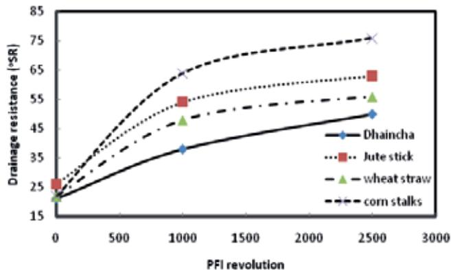
**Fig. 1. Increase of drainage resistance of KOH pulps with PFI revolution**
