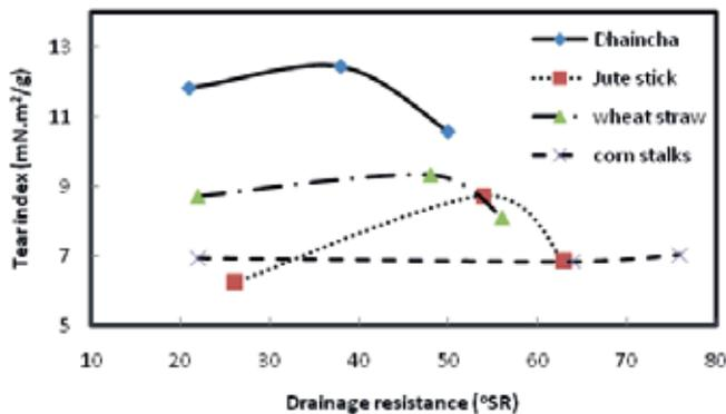
Fig. 3. Tear index development of KOH pulps with °SR
