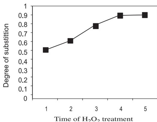
**Graph 5. Degree of substitution of CMC Vs time of H<sub>2</sub>O<sub>2</sub> treatment in hour**
