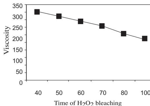
**Graph 6. Viscosity of CMC in cp Vs Time of H<sub>2</sub>O<sub>2</sub> treatment**
