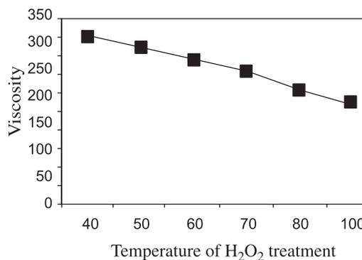
**Graph 8. Viscosity of CMC in cp Vs Temperature of H<sub>2</sub>O<sub>2</sub> treatment**
