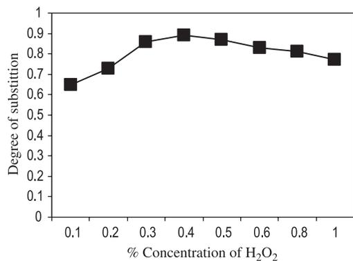
**Graph 1. Degree of substitution of CMC Vs Percentage of H<sub>2</sub>O<sub>2</sub> concentration**
