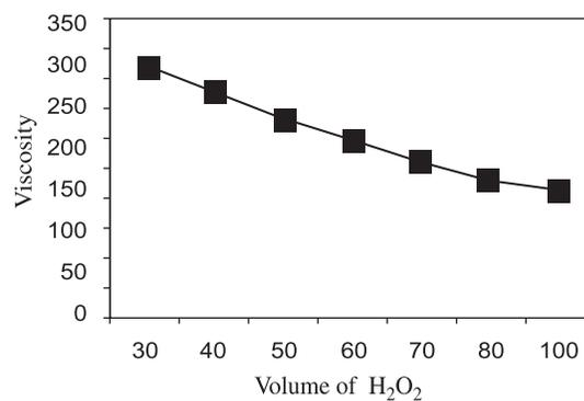
**Graph 4. Viscosity of CMC in cp Vs volume of H<sub>2</sub>O<sub>2</sub> liquor**
