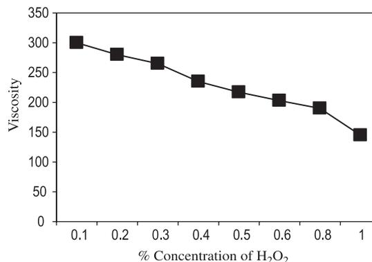
**Graph 2. Viscosity of CMC in cp Vs Concentration of H<sub>2</sub>O<sub>2</sub> of bleaching treatment**
