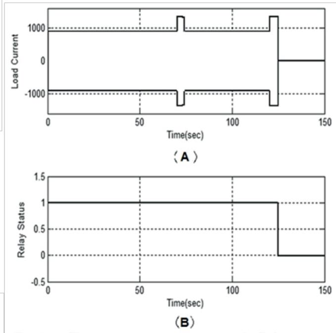
Fig. 8. (a) The generator output current, (b) Relay status
