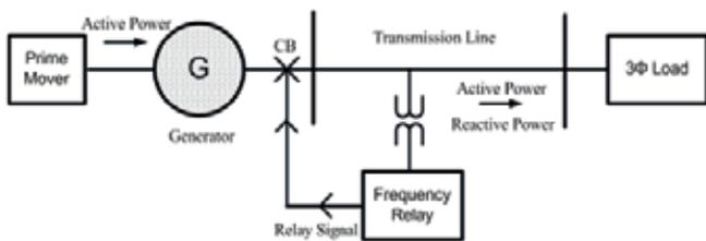
**Fig. 1. The location of the frequency relay**
