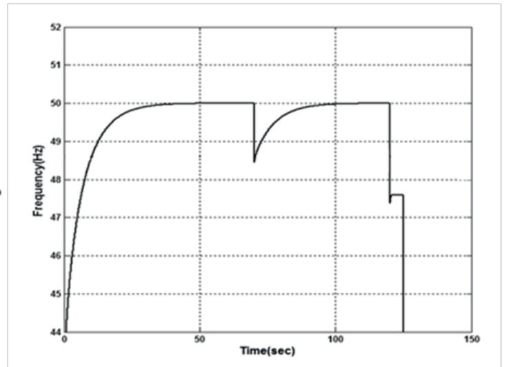
Fig. 5. The grid frequency curve while adding charges
