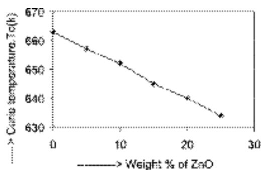
Fig. 2.6. Composition dependent  $T_c$  in Mn-Zn ferrite (Group B samples)
