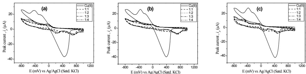
**Fig. 7.** CVs of Cu(II) (solid), and Cu(II)/Rab with different ratio (i) 1:1 (dash), (ii) 1:2 (dot), (iii) 1:3 (dash dot), and (iv) 1:4 (dash dot dot) in acetate buffer solution at (a) pH 3.5, (b) pH 4.0 and (c) pH 4.5
