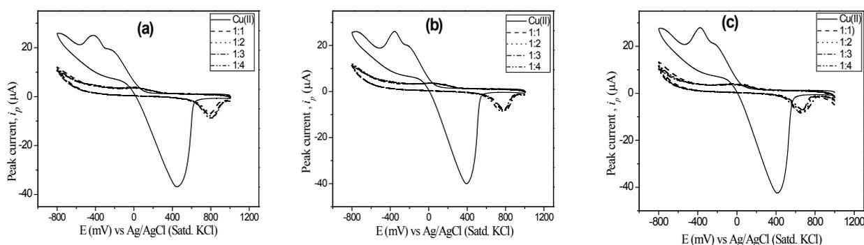
**Fig. 5.** CVs of Cu(II) (solid), and Cu(II)/Pan with different ratio (i) 1:1 (dash), (ii) 1:2 (dot), (iii) 1:3 (dash dot), and (iv) 1:4 (dash dot dot) in acetate buffer solution at (a) pH 3.5, (b) pH 4.0 and (c) pH 4.5.
