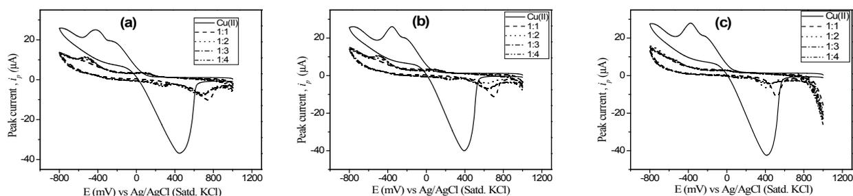
**Fig. 6.** CVs of Cu(II) (solid), and Cu(II)/Eso with different ratio (i) 1:1 (dash), (ii) 1:2 (dot), (iii) 1:3 (dash dot), and (iv) 1:4 (dash dot dot) in acetate buffer solution at (a) pH 3.5, (b) pH 4.0 and (c) pH 4.5.
