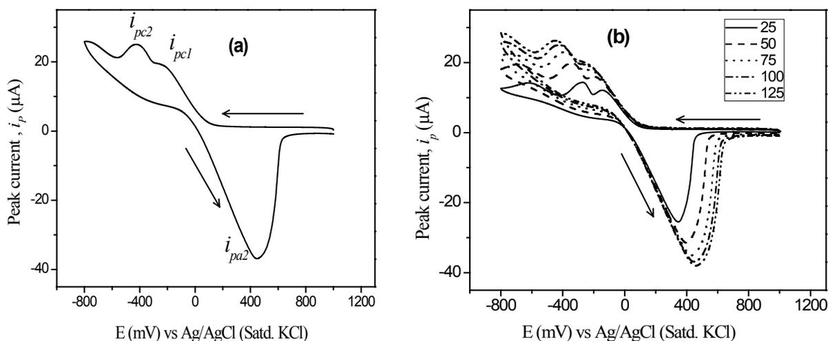
**Fig. 1. (a) CV of  $1.0 \text{ mM Cu(II)}$  in acetate buffer solution at pH 3.5 with scan rate of  $100 \text{ mVs}^{-1}$  and (b) CVs of  $1.0 \text{ mM Cu(II)}$  at various scan rate: 25 (solid), 50 (dash), 75 (dot), 100 (dash dot), and 125 (dash dot dot)  $\text{mVs}^{-1}$  at GCE.**
