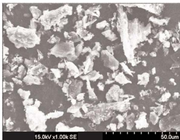
**Fig. 3.** SEM image of activated charcoal
