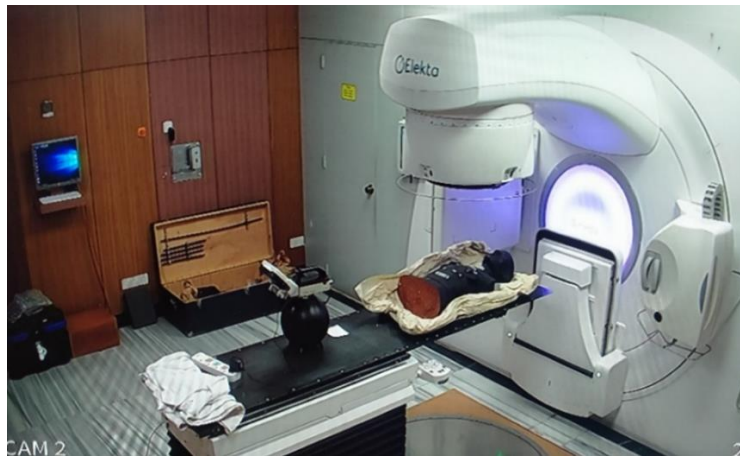
Fig. 4: Camera view during irradiating TLDs in 15 MV Linac (Elekta type) in Enam Medical College & Hospital, Savar, Bangladesh.
