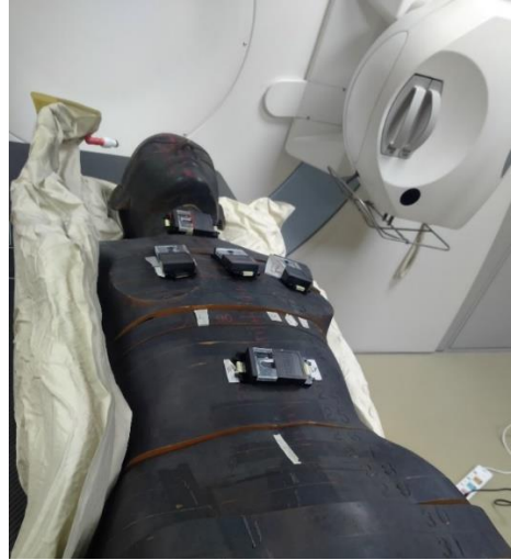
Fig. 3: TLD set up on Alderson Rando phantom placed on the Linac treatment couch.
