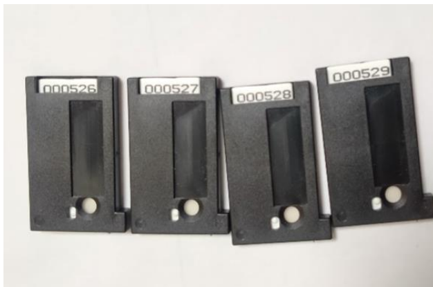
Fig. 1: TL crystals inside card holder.
