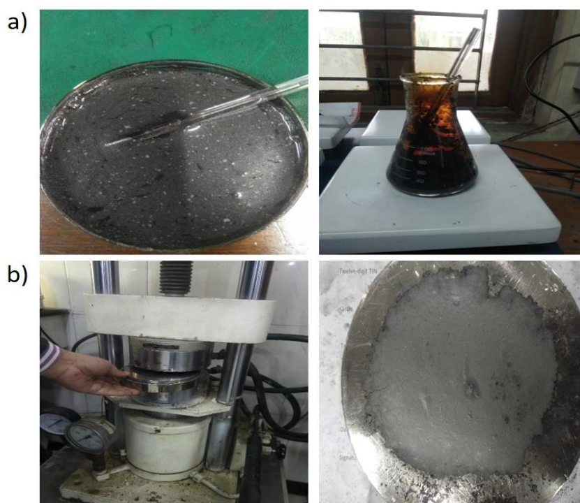
Fig. 1. Preparation and molding process of GO. (a) Pretreating Graphite powder with a mixture of Sulfuric acid and Nitric acid, and (b) Forming Graphite sheets using PVA as a binder.
