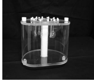
Fig. 3: NEMA Image quality body phantom (Data Spectrum Inc., Durham, NC)
