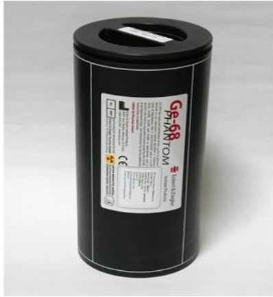
Fig. 2a: Ge-68 Annulus Phantom for Normalization
