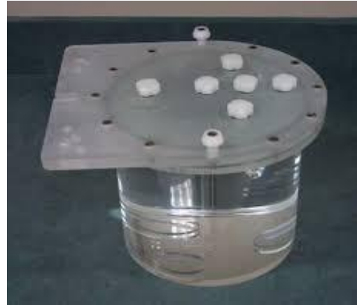
Fig. 2b: Cylindrical water phantom for Well Counter Correction
