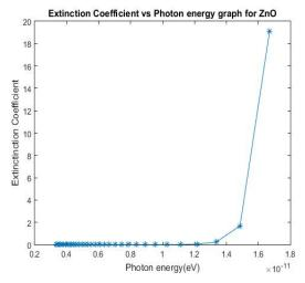
Fig. 3. Variation of extinction coefficient as a function of photon energy for ZnO thin film.
