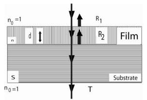
Fig. 1: Model of the thin absorbent films on a transparent thick substrate [15]
