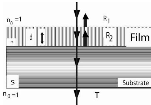
Fig. 1: Model of the thin absorbent films on a transparent thick substrate [15]
