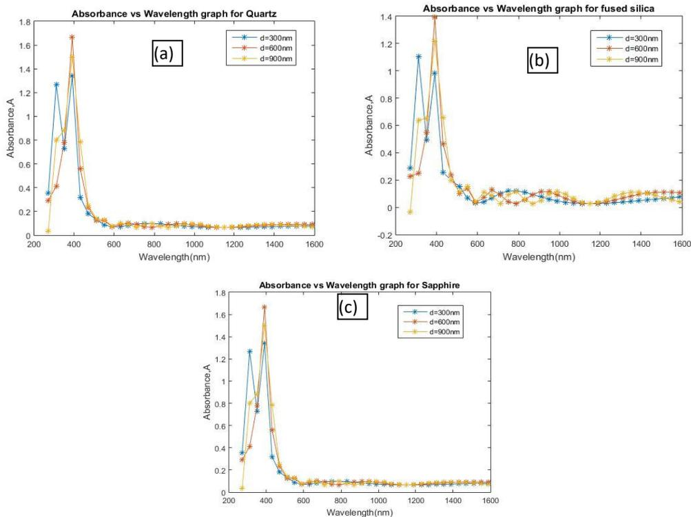
**Fig. 6.** Absorbance spectra of ZnO thin film for different thicknesses deposited on (a) Quartz (b) Fused Silica and (c) Sapphire substrates.
