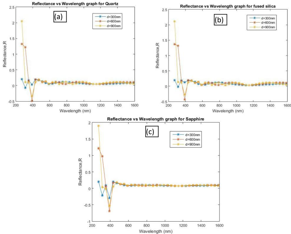
**Fig. 5.** Reflectance spectrum of ZnO thin film for different thicknesses deposited on (a) Quartz (b) Fused silica and (c) Sapphire substrate.
