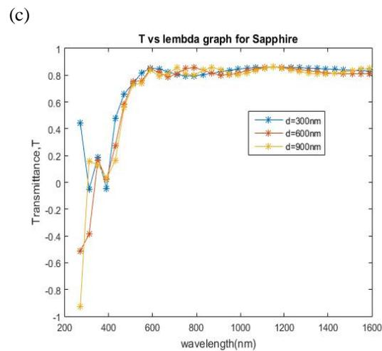
**Fig. 4.** Transmission spectra of ZnO thin film for different thicknesses deposited on (a) Quartz (b) Fused silica and (c) Sapphire substrates.
