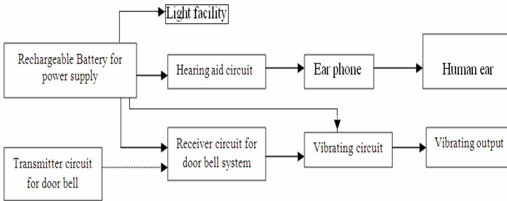
**Figure 3:** Block Diagram and Its brief description of the low cost multi use hearing aid.
