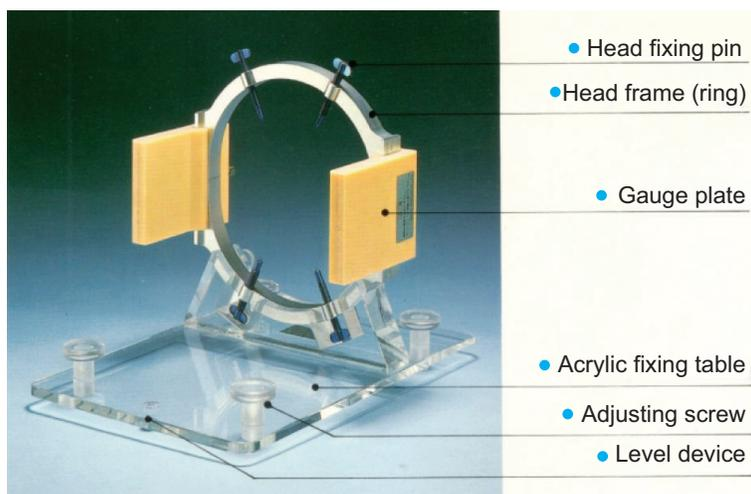
**Fig.-2: Basic setting for a "KOMAI" frame system**
