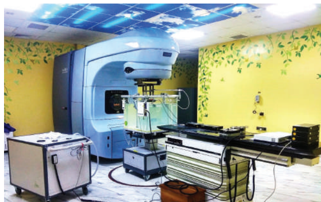
Figure 1: Dosimetric Setup for Small Field Dosimetry at INMP
