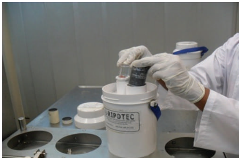
Figure 1: Collection of eluates from the RIPDTEC Mo-99/Tc-99m chromatographic column generator
