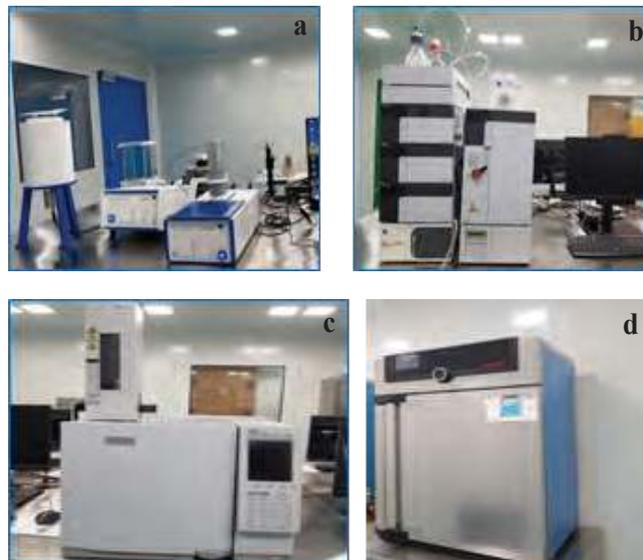
Figure 3: a) Raytest Mucha (Gamma Spectrometer) & mini Gita (Radio-TLC scanner) b) Radio-HPLC c) Gas Chromatography d) Drying, heating oven for Sterility test.
