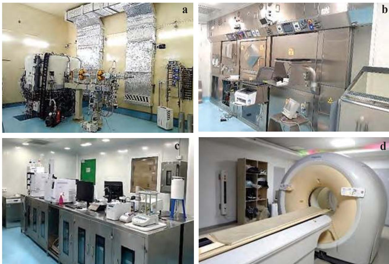
Figure 1: a) Recent view of 18/9 MeV Cyclotron, IBA S. A., Belgium b) Hot cells for synthesis and dispensing c) Quality control room d) Philips Ingenuity TF PET/CT
