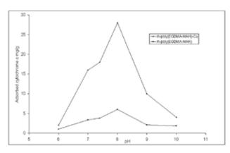
Fig.2. pH effect on adsorption capacity.
