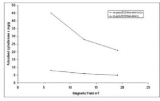
Fig.6. Magnetic field effect on adsorption capacity.
