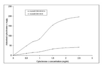
Fig.3. Cyt c concentration effect on adsorption capacity.
