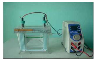
Figure 1: Polyacrylamide gel electrophoresis Chamber
