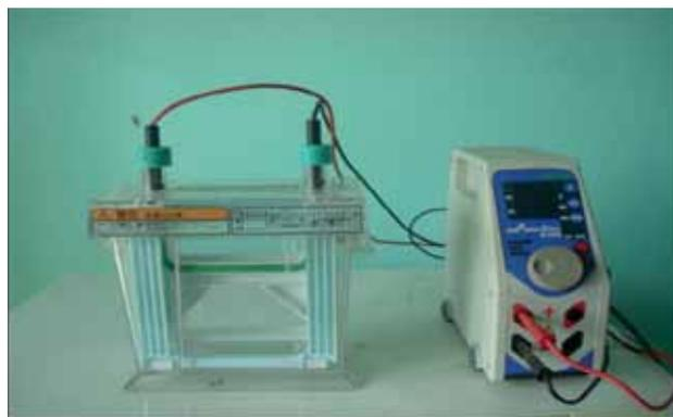
Figure 1: Polyacrylamide gel electrophoresis Chamber
