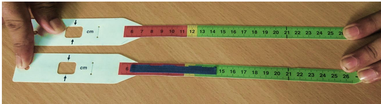
Fig. 3: Elastic band stretched just to touch the MUAC strap in the CT-MUAC device (front). The conventional device is shown at the back
