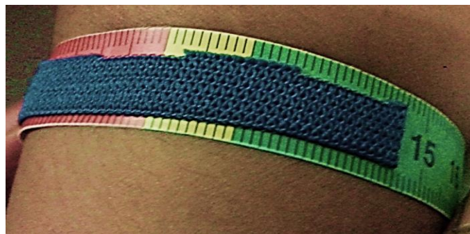
Fig. 4: Elastic band stretched just to touch the MUAC strap in the CT-MUAC device while taking measurements on human subjects
